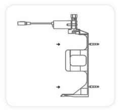
5. Assemble the tube from the pump to the soap dispenser.
